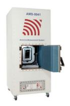
ETS-Lindgren's AMS-8041 is a self-contained enclosure for making wireless device over-the-air performance and passive antenna pattern measurements. The unit is ideal for design verification, pre-certification, production sample, desense, and regression testing.
